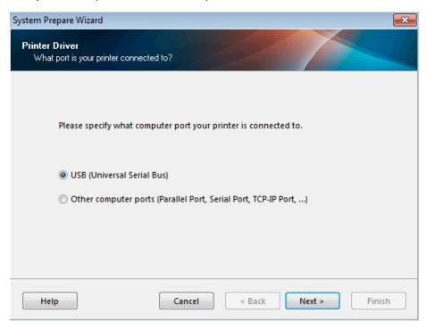
11. Insert a new roll of labels into your Zebra printer. Connect one end of the supplied USB cable to the Zebra printer and the other end to your local computer. Power the Zebra printer on and click **Finish**. Windows will now install the printer, which can be located and verified by clicking the **Start** button and selecting **Devices and Printers**.
